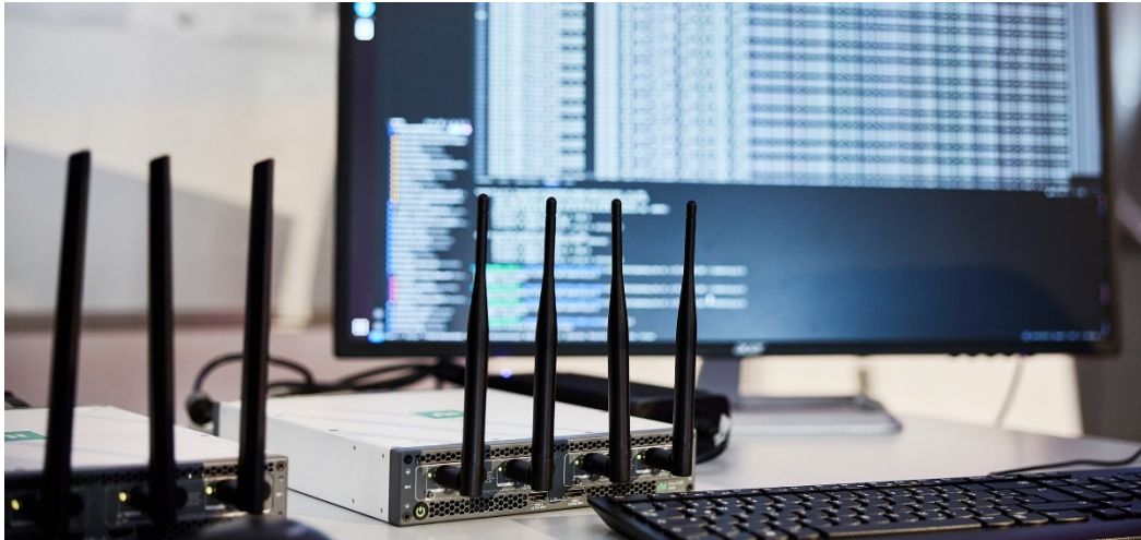
Software-defined radio, DECT NR+ demonstrator developed by Leibniz University Hanover
